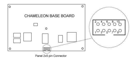
This connector is a standard 2x5 IDC 2,54mm socket. The signals for each pin are the following:
