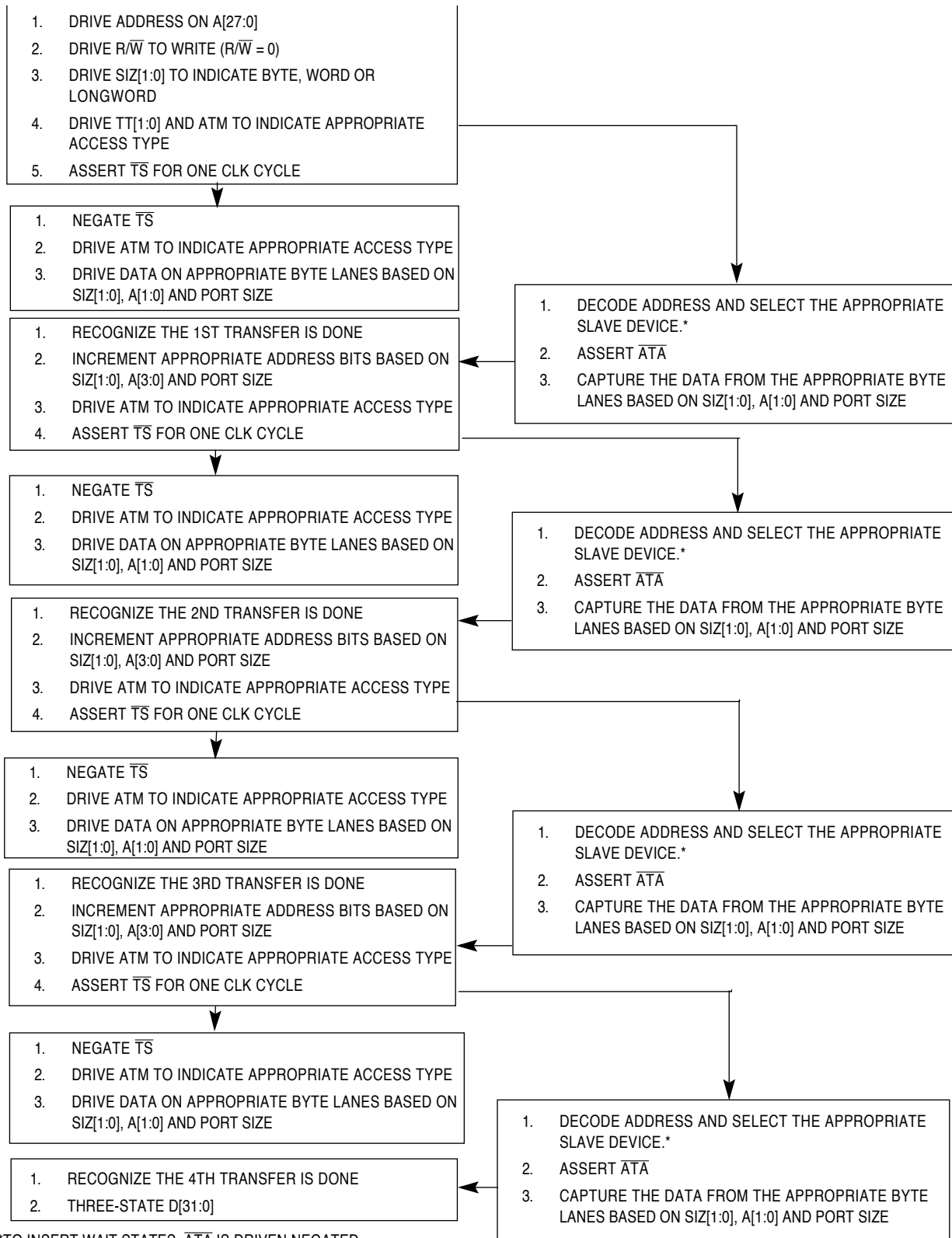
Figure 6-26. Burst-Inhibited Word-, Longword-, and Line-Write Transfer with Asynchronous Termination Flowchart
